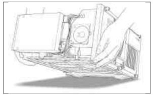
Laying the computer on its side for easy access
